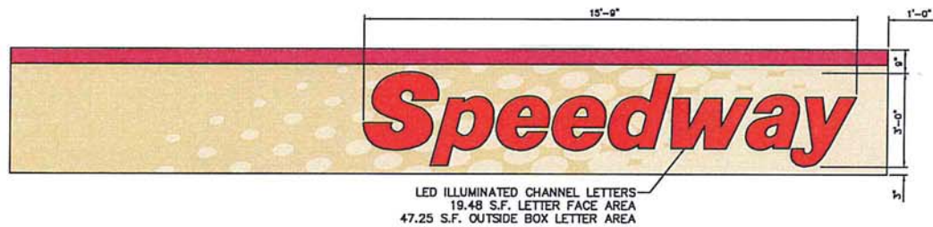
B FRONT LEFT AUTO CANOPY FASCIA SIGNAGE ELEVATION 3994-SS1 SCALE: NOT TO SCALE
