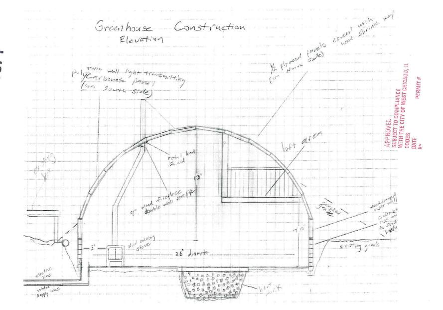
Greenhouse Construction floor plan Geodesic Pisci wall 2x6 dome frame covered with plywood and polycarbonate Panels
