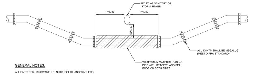
ASSOCIATED WITH THE WATERMAIN AND CASING SPACERS SHALL BE STAINLESS STEEL.
